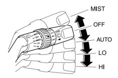
Turn the wipers on by pulling the lever down. AUTO — Auto control LO — Low speed
